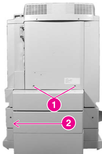
Figure 6-3. Removing and replacing the rear cover
